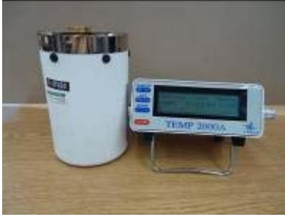
We can also test total hemispherical emittance ( $\epsilon_H$ ) on the AZ Technology Temp 2000A. A calculated hemispherical value can be provided by testing on the AZ Technology Temp 2000A Reflectometer in the Relative Mode. Because the ASTM-E-408 Method B specifically calls out testing on an emissometer and not a reflectometer, this alternative method will not technically meet ASTM-E408 Method B.
