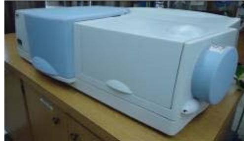
Multek measures solar absorptance using a Perkin-Elmer Labsphere 950 UV-VIS-NIR spectrophotometer.
