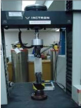
All tapes sold by Multek are tested for bond strength. This test is done by applying the tape to a clean stainless steel substrate using a prescribed pressure and then measuring the force required to remove the tape using an Instron instrument. Our test methodology is in accordance with ASTM D-1000 and ASTM D-3330. We can also test adhesion to aluminum plates if desired.
