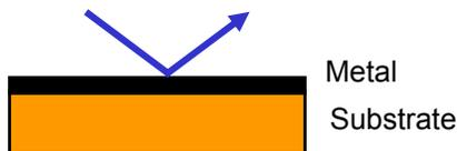
A first surface mirror consists of a metallic coating (typically aluminum or gold) on a substrate. For multilayer insulation (MLI) blankets the substrate is usually PET or polyimide film, though FEP is used in some applications. Metallic coatings have very low emittance, so films coated on both sides are typically used for the inner layers of insulation blankets to minimize heat transfer.
