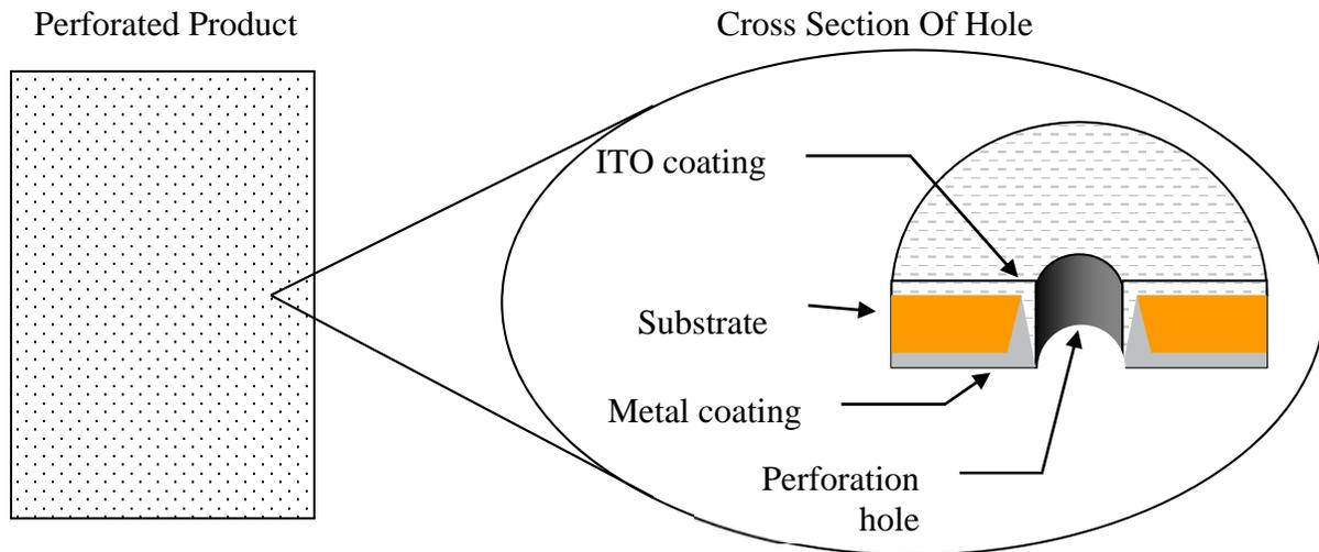
**Figure 1 Perforated interconnections**
